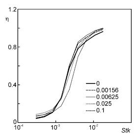
Figure 15. Grade efficiency curves for various mass loadings ( $\phi_{\rm m}=$  0: one-way coupled,  $\phi_{\rm m}>$  0: two-way coupled).
