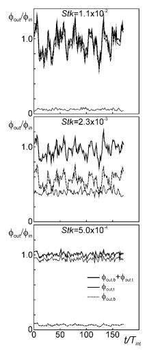
Figure 6. Quasi-steady-state time series of the particle flux through the top and bottom exhaust surfaces for three different particle sizes/Stokes numbers for a one-way couples simulation (Case 1).
