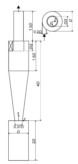
Figure 5. Flow geometry and coordinate system of the Stairmand cyclone: left: side view, right: top view.
