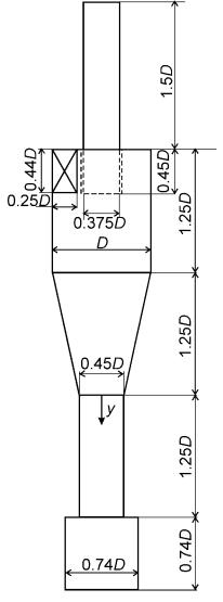
Figure 1. Cyclone geometry due to Obermair et al. <sup>18</sup>
