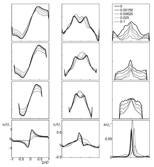
Figure 11. Radial profiles of the time averaged gas flow under various mass loading conditions ( $\phi_{\rm m}=0$ : one-way coupled,  $\phi_{\rm m}>0$ : two-way coupled).
