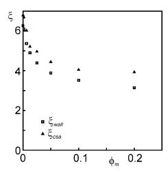
Figure 13. Pressure drop coefficient as a function of the mass loading.
