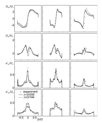
Figure 2. Radial profiles of the tangential and axial velocity at three axial levels in the Obermair et al.  $^{17,18}$  cyclone at  $Re = 3.4 \cdot 10^5$ .
