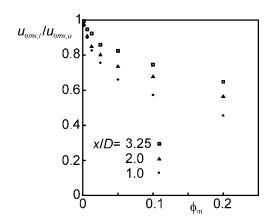
Figure 12. Decay of the swirl velocity in terms of the ratio of the maximum swirl velocity under loaded  $(u_{\theta mx,l})$  and unloaded  $(u_{\theta mx,u})$  conditions as a function of mass loading for three axial levels in the cyclone.
