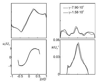
Figure 18. Swirl and turbulent kinetic energy profiles at x/D=3.25 (top), and 1.0. Sensitivity with respect to the number of particles per parcel  $\gamma$ . Two-way coupled simulations with  $\phi_{\rm m}=0.1$  (cases 8 and 9).
