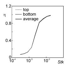
Figure 14. Grade efficiency for the two-way coupled simulation with  $\phi_{\rm m}=$  0.0125 (Case 5) as measured through the top, the bottom and the average of these two.
