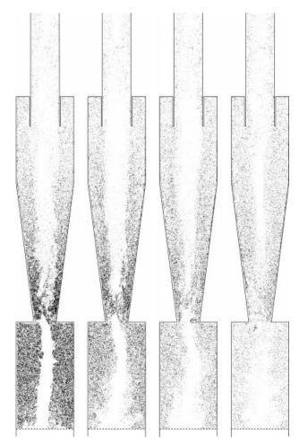
Figure 8. Instantaneous realizations of the particles with  $Stk = 2.3 \cdot 10^{-3}$  in vertical slice, with thickness of 0.02D through the center of the cyclone (the xy-plane) in (from left to right) a one-way coupled simulation, and two-way coupled simulations with mass-loading 0.00625, 0.025, and 0.1, respectively.
